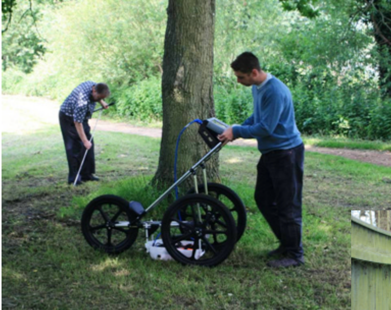
Ground Penetrating Radar using automated cart to locate tree roots
